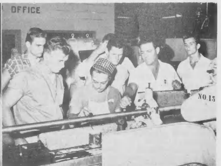
THE STUDENTS get a demonstration of the workings of a cylinder grinder machine which is reconditioning a worn pump shaft to standard size. Operator is Juancinto Kock.
